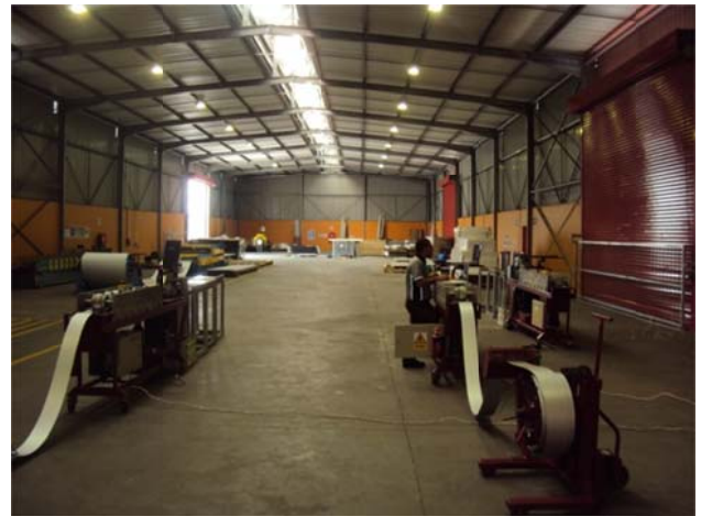
Factory set up with 3 SCS 63mm rollformers
