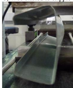
d) Ultimate failure
