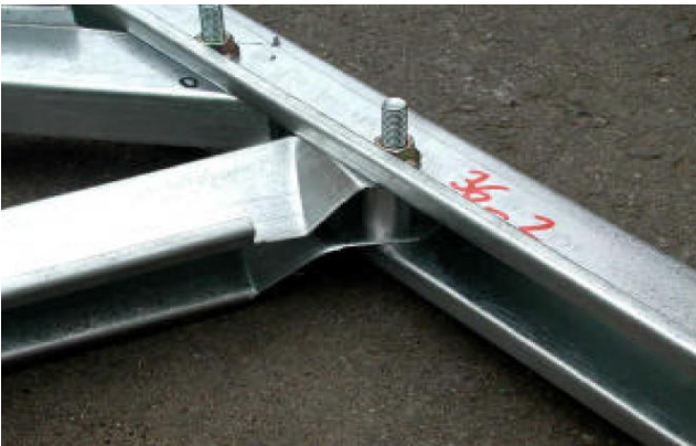
Hat section roof truss connection tests
