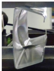
b) Web started to cripple
