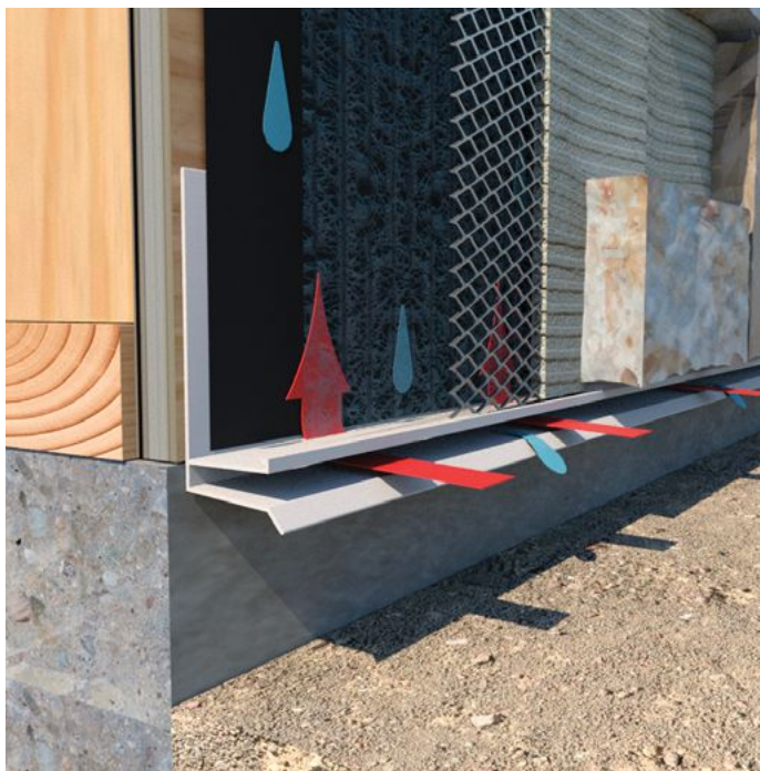
Shown is ClarkDietrich's Drip Flashing for Rainscreen (left), with interstitial space to permit termination of the cladding system above while allowing draining and ventilation. The Top Vent Track (right) creates alignment for the Drain Mat, providing a space for the mat to vent and dry via convective air flow from the DFLRS on the bottom.
