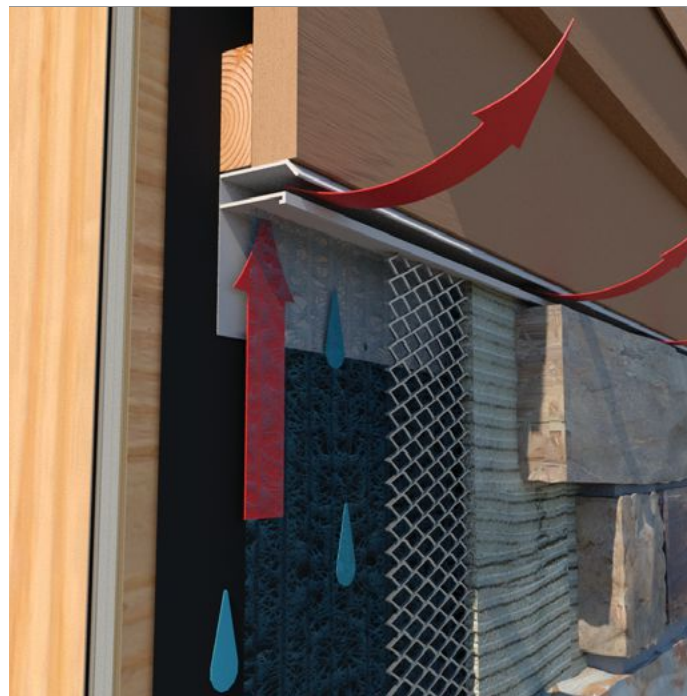
Shown is ClarkDietrich's Drip Flashing for Rainscreen (left), with interstitial space to permit termination of the cladding system above while allowing draining and ventilation. The Top Vent Track (right) creates alignment for the Drain Mat, providing a space for the mat to vent and dry via convective air flow from the DFLRS on the bottom.
