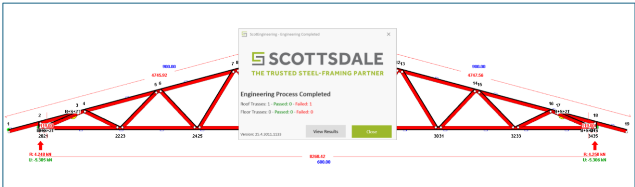
Figure 19 - Truss with failed status
