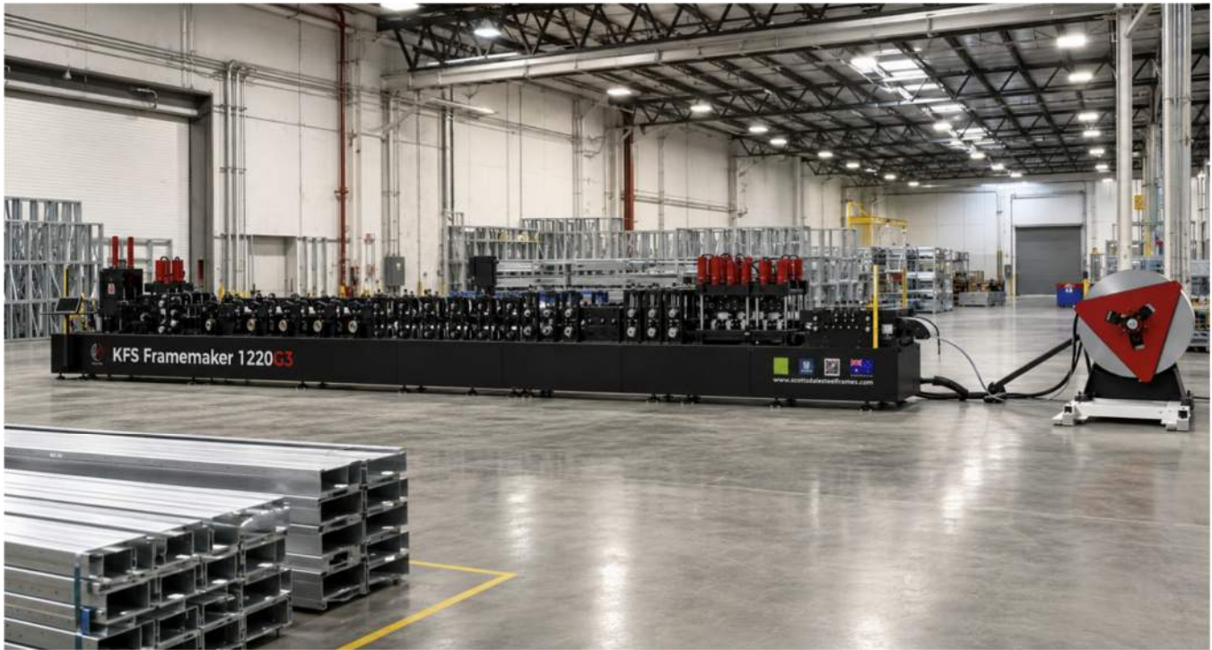
Figure 14 KFS Framemaker 1220G3 inside a large framing factory
