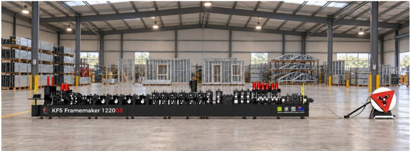
Figure 1 KFS Framemaker 1220G3 and decoiler in a light-gauge steel framing shop
