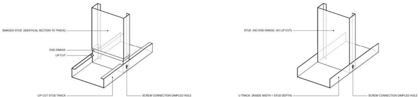
Figure 2 The Panelizer and the Hybrid Mode Methods of LGS Fabrication
